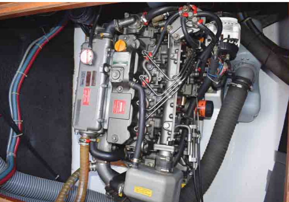
ABOVE LEFT: Trusty Yanmar 50hp diesel.
